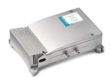
2-input (VHF+UHF, SAT) indoor amplifier with 40dB gain and up to  $125dB\mu V$  output level on SAT band, gain adjustment (20dB) and low noise figure.
