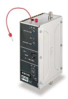
Wideband amplifiers with push-pull technology capable of amplifying the entire 47-862 MHz band. Equipped with one input and one output, they are used to amplify the signal coming from a KF filter battery or other modules (receivers, modulators, etc.).
