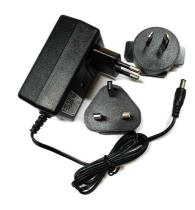
**12V 2A** power supply with **Male Jack connector** (2.5x5.5x12; inside positive, outside negative) and **adaptors** for standard **plugs of different countries**.
