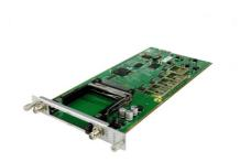
**GX-4S2CI-BP-01** module is equipped with two RF coaxial Satellite inputs and two PCMCIA Common Interface slots. The module is able to tune up to **four DVB-S/S2/S2X satellite transponders** (two transponders for every single RF coaxial input), decrypt the scrambled programs through the C.I. slots and share and pool the contents to the **GALAXIA** main chassis.
