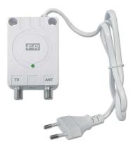
12V stabilized switching type power supply with high efficiency and low consumption with 1 input, 1 output and 400mA delivered current. C-type plug for mains connection.
